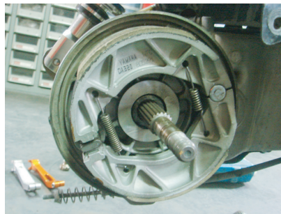
8. 裝回煞車皮 INSTALL BRAKE SHOE.
