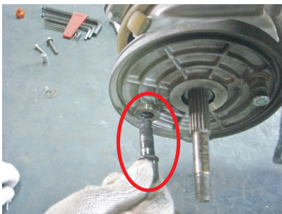
7. 裝回原車煞車臂桿 INSTALL ORIGINAL BEARING ROD.
