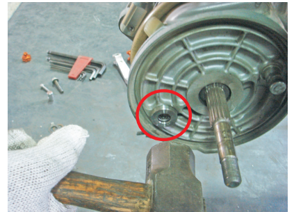
6. 以鐵鎚敲入培林套管 LIGHTLY BEAT BEARING BUSH INSIDE.
