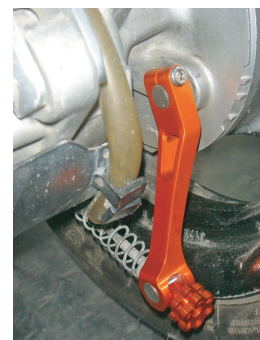
9. 安裝加長煞車搖臂，調整適當角度用六角板手鎖緊 INSTALL LONGER BRAKE REAR ARM AND THEN ADJUST THE ANGLE. FINALLY USE RATCHETING WRENCH TO LOCK WELL.
