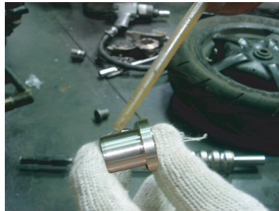
5. NCV專利培林套管，安裝前抹上少許機油，方便安裝 PLEASE ADD SOME ENGINE OIL BEFORE INSTALLING BEARING.
