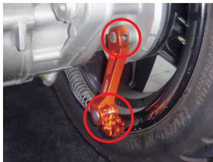
7. INSTALL LONGER BRAKE REAR ARM AND THEN ADJUST THE ANGLE. FINALLY USE RATCHETING WRENCH TO LOCK WELL, INSTALL BRAKE ADJUST SCREW WELL.
