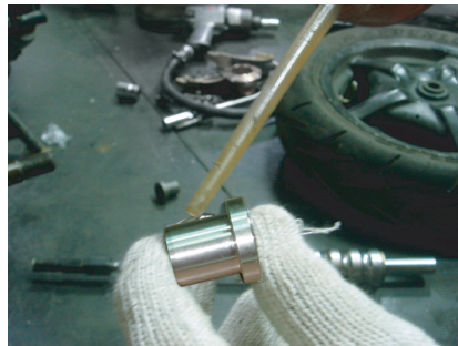
5. PLEASE ADD SOME ENGINE OIL BEFORE INSTALLING BEARING.
