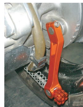
9. INSTALL LONGER BRAKE REAR ARM AND THEN ADJUST THE ANGLE. FINALLY USE RATCHETING WRENCH TO LOCK WELL.
