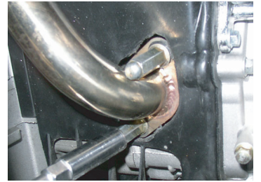
3. LOCK IT WELL WITH EXHAUST PIPE SCREW
