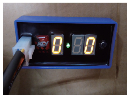
9.TURN ON THE SWITCH. IF LIGHT IS ON, THAT MEANS THE INSTALLATION IS CORRECT. USE VELCRO TO ATTACH THE ADJUSTER IN THE LUGGAGE BOX. (ADJUSTING EXPLANATION ON PACKAGE)
