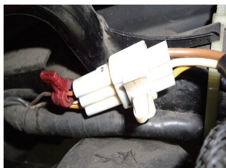
7.MAKE ELECTRIC WIRE CLIP CONNECT TO ALTERNATOR SIGNAL WIRE (BROWN)
