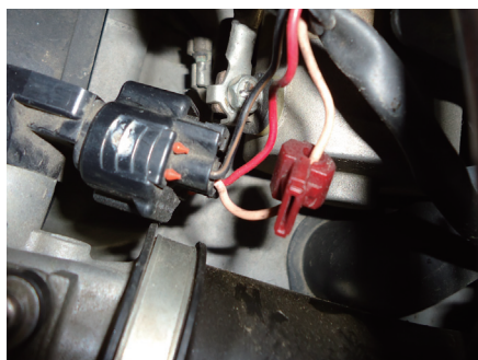
5.MAKE ELECTRIC WIRE CLIP CONNECT TO TPS SIGNAL WIRE (PINK)
