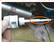
檢查機油尺油量是否到達標準刻度 並酌量加入機油 CHECK THAT WHETHER OIL LEVEL OF OIL LEVEL GAUGE REACHES STANDARD OR NOT AND THEN ADD OIL BY THE SITUATION.
