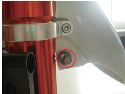
4. USE ORIGINAL FRONT FENDER SCREW TO LOCK FRONT FENDER AND FRONT FENDER RING. . AND THEN LOCK STEP NO. 2
