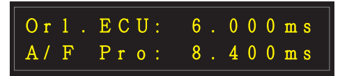
原廠供油時間 調整後供油時間 ORIGINAL OIL SUPPLY TIMING OIL SUPPLY TIMING AFTER ADJUSTING
