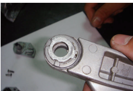
5.取出原廠腳踏桿背面之旋轉彈簧與彈簧護蓋。(取出時須注意旋轉彈簧置入的方向) Remove the rotating spring & spring cover from the back of original footrest rod. (notice the installing direction of rotating spring as removing.)
