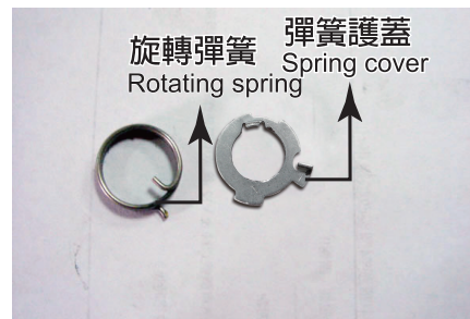
5.取出原廠腳踏桿背面之旋轉彈簧與彈簧護蓋。(取出時須注意旋轉彈簧置入的方向) Remove the rotating spring & spring cover from the back of original footrest rod. (notice the installing direction of rotating spring as removing.)
