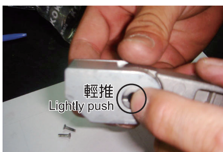
2.輕推腳踏桿背面基礎座上蓋軸心使上蓋與基座分離。(小心彈簧會彈出) Lightly push upper cover shaft of back footrest rod base to make upper cover and base separated. P.S. (be careful for pop-up spring)
