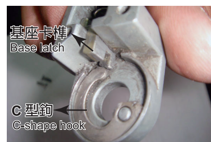
8.將基座本體的卡榫與C型鉤固定於相關位置如上圖。 Fix the base latch and c-shape hook into related position shown above photo.
