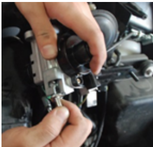
步驟6: 安裝行李箱及油箱蓋鋼索 STEP 6: INSTALL THE STEEL WIRE CONNECTING TO OIL TANK & LUGGAGE BOX.
