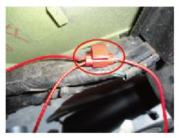
3. TURN ON SWITCH TO TEST WHICH WIRE IS (+) WITH ELECTRIC METER AND CONNECT TO THE RED WIRE (+) OF ADJUSTER.
