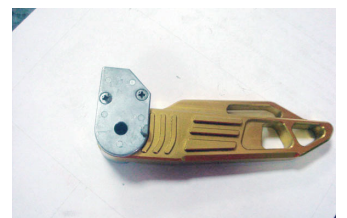
14. LOCK UPPER COVER WITH SCREWS AND CHECK IF THE MOVEMENT OF FOOTREST ROD SET WORKS NORMALLY. IF NOT, PLEASE FOLLOW STEP 7 AND INSTALL AGAIN.
