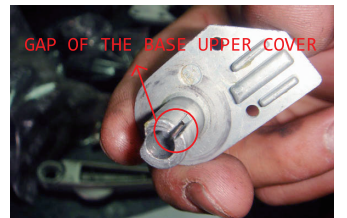
12. PUT THE RAISING POINT OF ROTATION SPRING INTO THE GAP OF THE BASE UPPER COVER.
