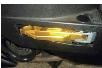
15. IF THE FOOTREST ROD SET WORKS NORMALLY, INSTALL IT ON THE SCOOTER DIRECTLY.
