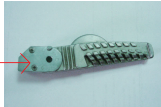
1. TAKE OFF ORIGINAL FOOTREST ROD SET FROM SCOOTER.
