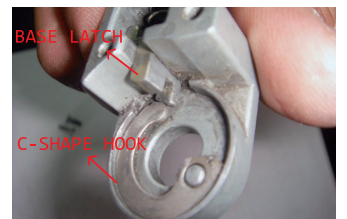
10. FIX THE BASE LATCH AND C-SHAPE HOOK INTO RELATED POSITION SHOWN ABOVE PHOTO
