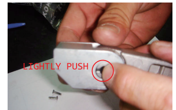
3. LIGHTLY PUSH UPPER COVER SHAFT OF BACK FOOTREST ROD BASE TO MAKE UPPER COVER AND BASE SEPERATED. PS. (BE CAREFUL FOR POP-UP SPRING)
