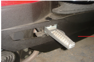
1. TAKE OFF ORIGINAL FOOTREST ROD SET FROM SCOOTER.
