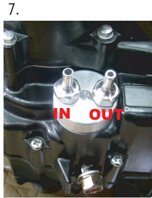
旋轉開 TAKE APART OIL PAN SCREW COVER
