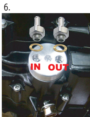
旋轉開 TAKE APART OIL PAN SCREW COVER
