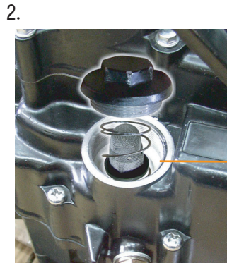
旋轉開 TAKE APART OIL PAN SCREW COVER
