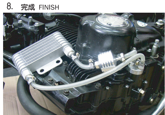
各個零件套上油管並用束環鎖緊即可 INSTALL OIL TUBE WITH EACH PARTS BY RING AND THEN LOCK WELL
