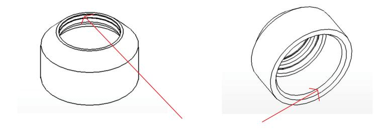
BEFORE INSTALLING IT, PLEASE ADD SOME OIL INSIDE TO MAKE INSTALLING EASILY.
