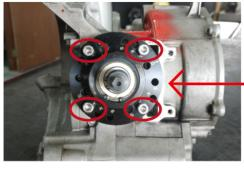
6. INSTALL CUTTING TOOL INTO ENGINE BODY AND LOCK SCREWS WELL.
