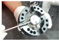
4. LOCK SCREWS OF CUTTING TOOL WELL.
