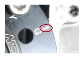
5. PLEASE NOTE THE UP **1** OF TOOL TOWARD CHAIN DIRECTION AS INSTALLING.
